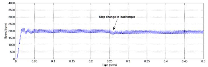
Fig.2 Drive response to change in reference change in load torque from no load to 0.125Nm
