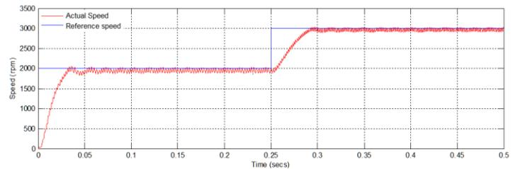
Fig.1 Drive response to change in reference speed from 2000rpm to 3000 rpm
